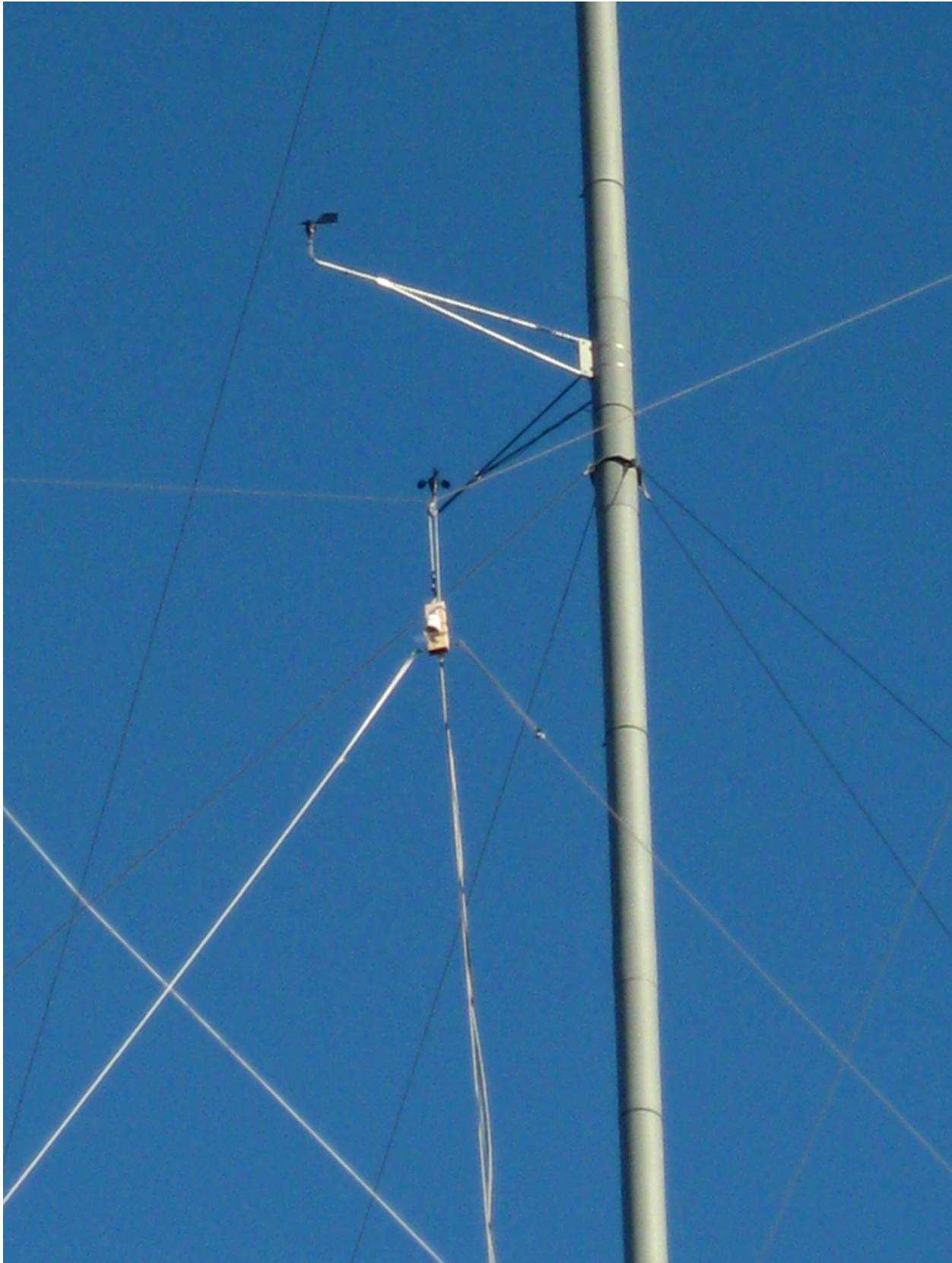
Photo A-3: The High microphone suspended in the cables of the met tower.
