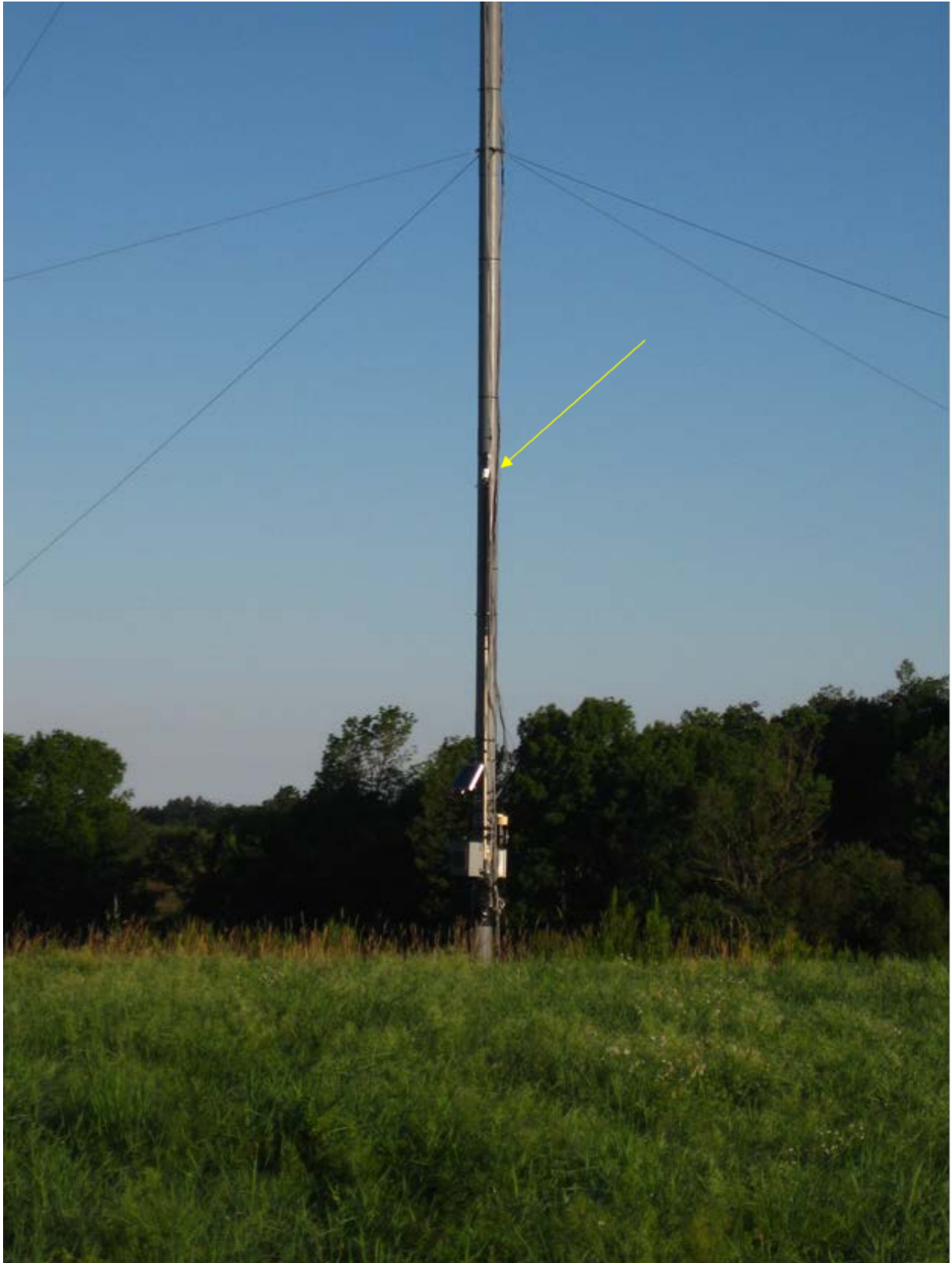
Photo A-1: Low microphone attached to the met tower.
