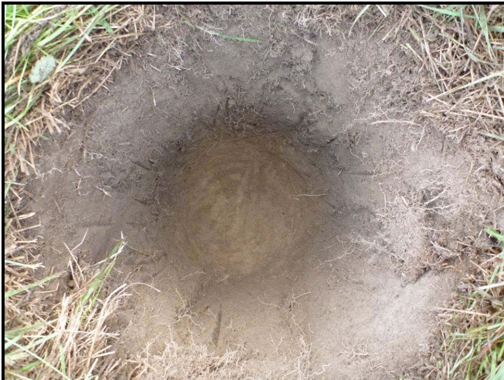
Image 10: View of Typical Test Pit Excavated into Subsoil near Known Watercourse (Photo Taken on July 13, 2011)
