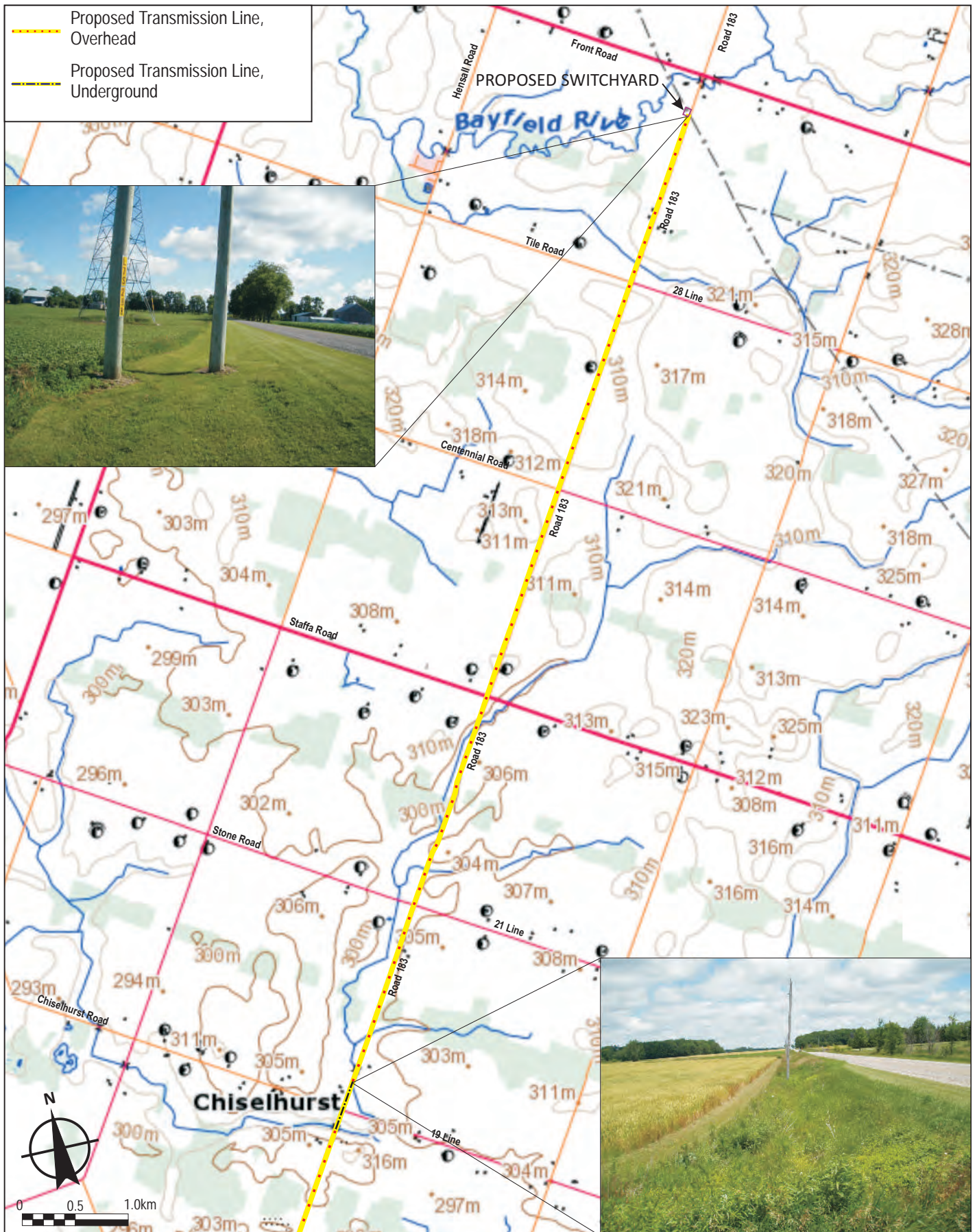
Figure 4 Eastern Portion of the Proposed 230kV Transmission Line
