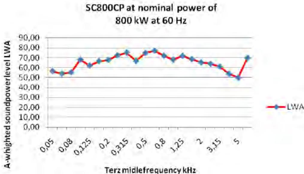
**Figure B.1** SC800CP Inverter Sound Power Level as Provided by SMA. Note that the Header in the Table above Represents Various Inverter Models of CS###CP Series.
