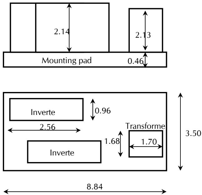
**Figure 3.1 Schematic Inverter Cluster Layout**
