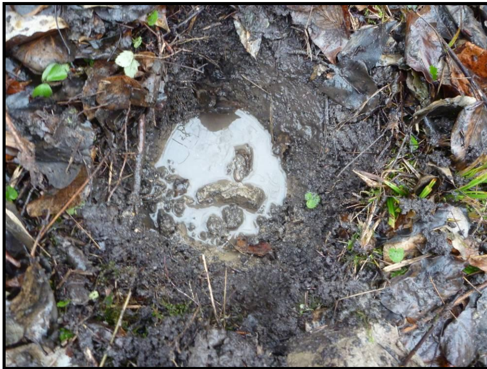
Plate 8: View of Typical Test Pit in Wet Area
