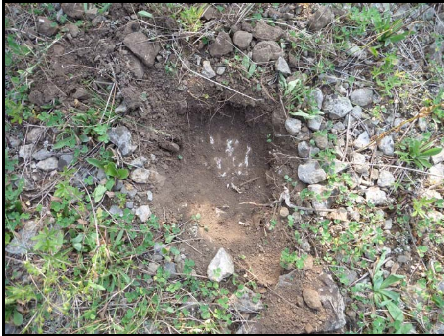
Plate 6: View of Test Pit in Gravel Fill, Excavated to Bedrock
