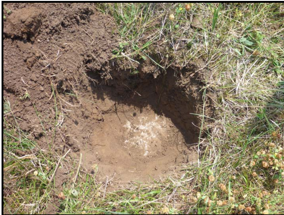
Plate 3: Typical Test Pit, Excavated to Bedrock
