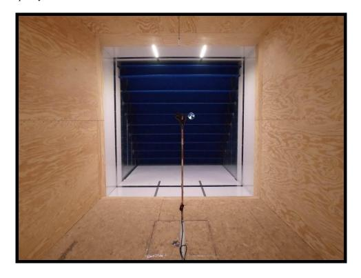
Photo of the wind tunnel setup. The cross-sectional area is  $2.5 \times 2.5 \text{ m}$ .
